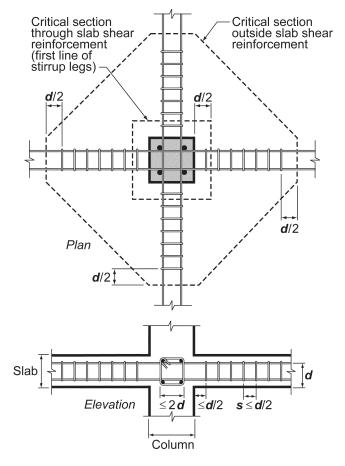
Fig.R8.7.6d—Arrangement of stirrup shear reinforcement, interior column.
