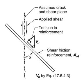
Fig. R22.9.4.3a—Tension in shear friction reinforcement.
