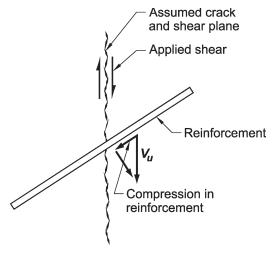
Shear-friction does not apply
