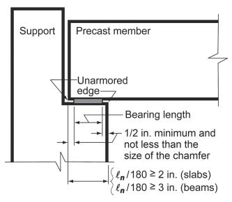
Fig. R16.2.6—Bearing length on support.
