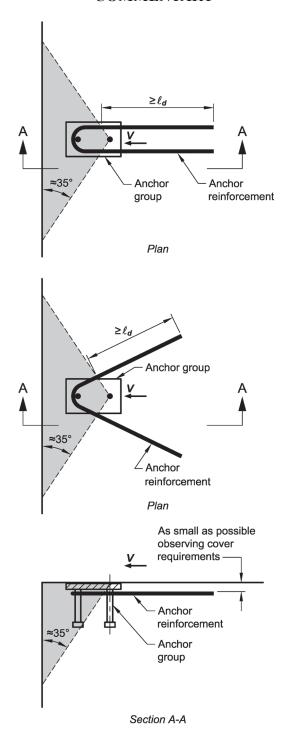
Fig. R17.5.2.9a—Hairpin anchor reinforcement for shear.
