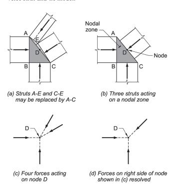
Fig. R23.2.2—Resolution of forces on a nodal zone.
