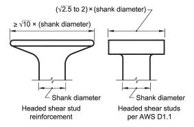
*Fig. R20.5.1*—Configurations of stud heads.
