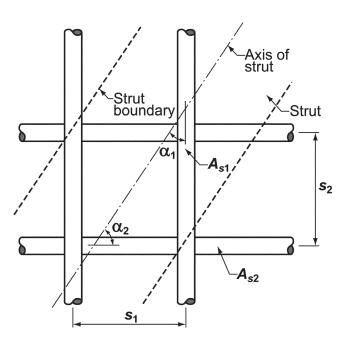
Fig. R23.5.3—Reinforcement crossing a strut.
