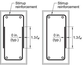
Fig. R25.7.1.7—Closed stirrup configurations.
