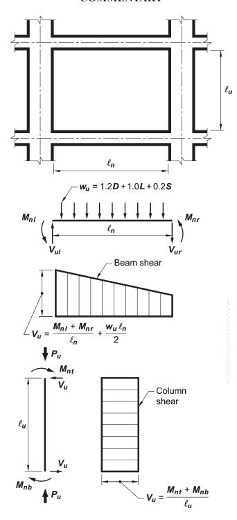
Fig. R18.4.2—Design shears for intermediate moment frames.
