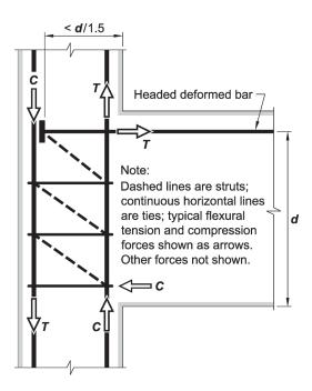
Fig. R25.4.4.2d—Breakout failure precluded in joint by providing transverse reinforcement to enable a strut-and-tie mechanism.
