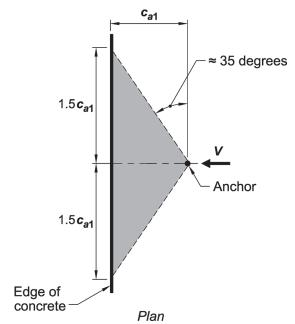
Fig. R17.3.2b—Breakout cone for shear.
