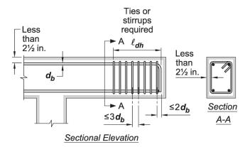
Fig. R25.4.3.3—Concrete cover according to 25.4.3.3.
