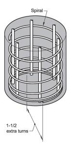
Fig. R25.7.3.4—Spiral anchorage.
