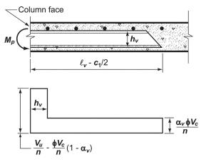
Fig. R22.6.9.6—Idealized shear acting on shearhead.
