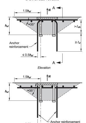
Fig. R17.4.2.9—Anchor reinforcement for tension.
