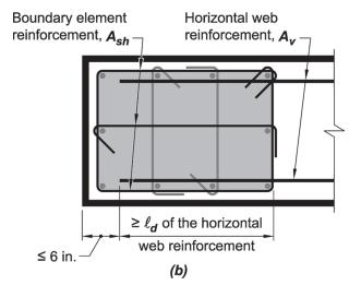
Option with straight developed reinforcement
