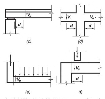
Fig. R9.4.3.2(c), (d), (e), (f)—Typical support conditions for locating factored shear force  $V_{\rm u}$ .
