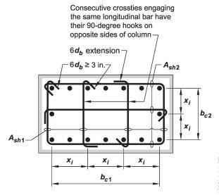
The dimension  $x_i$  from centerline to centerline of laterally supported longitudinal bars is not to exceed 14 inches. The term  $h_x$  used in Eq. (18.7.5.3) is taken as the largest value of  $x_i$ .
