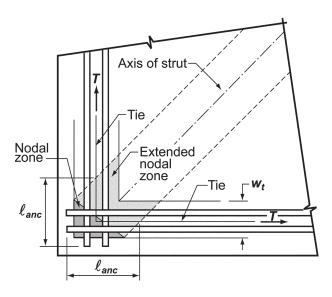
Fig. R23.8.2—Extended nodal zone anchoring two ties.
