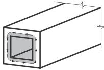
(b) Area enclosed by shear flow path
