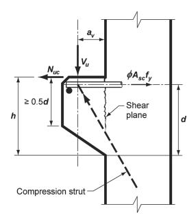
Fig. R16.5.1a—Structural action of a corbel.
