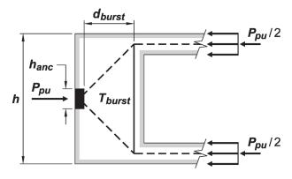
(b) <u>Flanged section with end diaphragm</u>  $T_{burst} \approx 0.50 P_{pu}$
