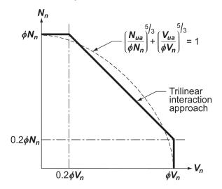
Fig. R17.6—Shear and tensile load interaction equation.
