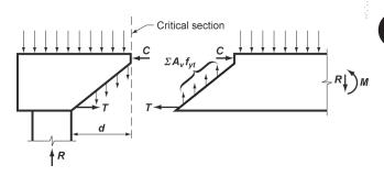
Fig. R9.4.3.2a—Free body diagrams of the end of a beam.
