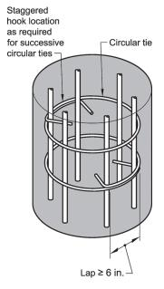
Fig. R25.7.2.4—Circular tie anchorage.
