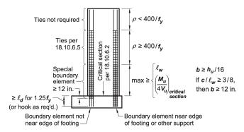
(a) Wall with  $h_W \ell_W \ge 2.0$  and a single critical section controlled by flexure and axial load designed using 18.10.6.2, 18.10.6.4, and 18.10.6.5
