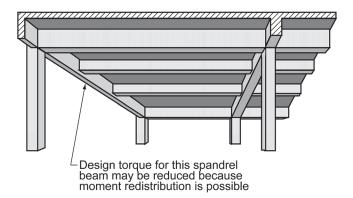
Fig. R22.7.3b—Compatibility torsion, the design torsional moment may be reduced (22.7.3.2).
