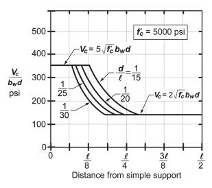
**Fig. R22.5.8.2**—Application of Table 22.5.8.2 to uniformly loaded prestressed members with  $f_c' = 5000$  psi.
