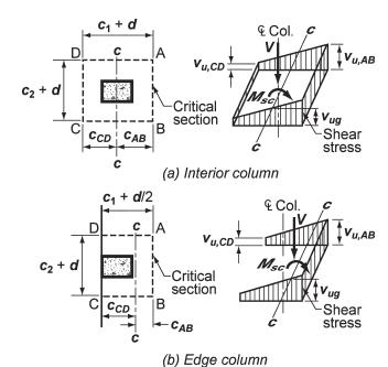
Fig. R8.4.4.2.3—Assumed distribution of shear stress.
