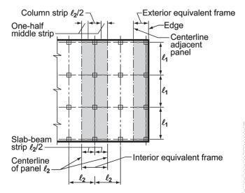
Fig. R8.11.2—Definitions of equivalent frame.
