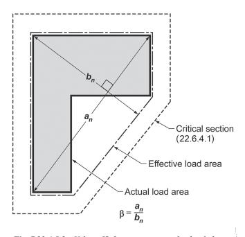
*Fig. R22.6.5.2*—*Value of*  $\beta$  *for a nonrectangular loaded area.*
