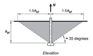
Fig. R17.3.2a—Breakout cone for tension.
