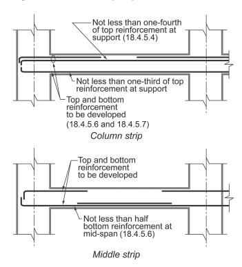
Fig. R18.4.5.3—Arrangement of reinforcement in slabs.
