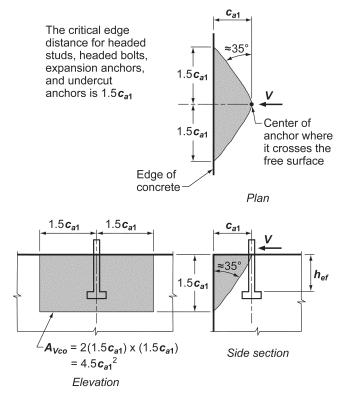
Fig. R17.5.2.1a—Calculation of A<sub>Vco</sub>
