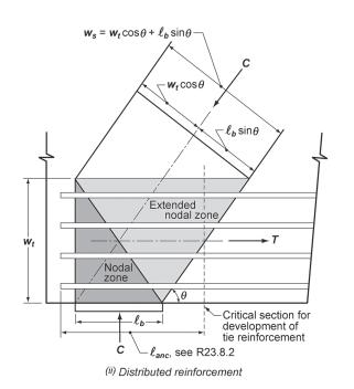
Fig. R23.2.6b—Extended nodal zone showing the effect of the distribution of the force.
