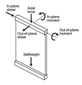
Fig. R11.4.1.3—In-plane and out-of-plane forces.
