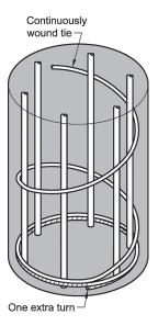
Fig. R25.7.2.3b—Continuous tie anchorage.
