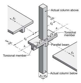
Fig. R8.11.4—Equivalent column (column plus torsional members).
