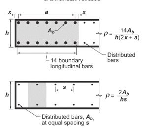
Fig. R18.10.6.5—Longitudinal reinforcement ratios for typical wall boundary conditions.
