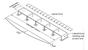
Fig. R12.4.2.3a—Example of diaphragm that might not be considered rigid in its plane.
