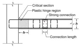
(a) Beam-to-beam connection
