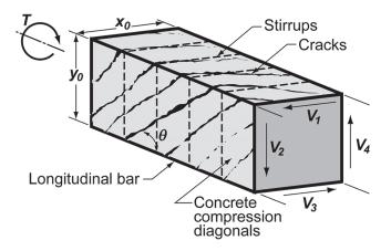
Fig. R22.7.6.1a—Space truss analogy.
