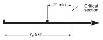
**Fig. R25.4.7.2**—Development of welded plain wire reinforcement.
