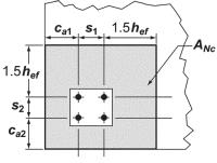
$$A_{Nc} = (c_{a1} + s_1 + 1.5h_{ef})(c_{a2} + s_2 + 1.5h_{ef})$$
