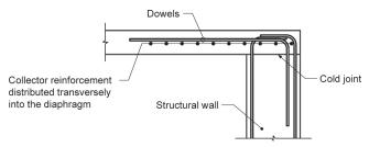
Fig. R12.5.3.7—Typical detail showing dowels provided for shear transfer to a structural wall through shear-friction.
