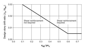
*Fig. R18.14.5.1*—*Illustration of the criterion of 18.14.5.1.*
