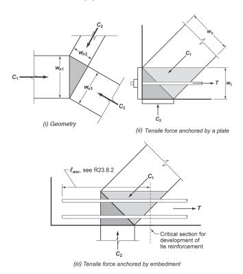
Fig. R23.2.6a—Hydrostatic nodes.
