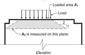
*Fig. R22.8.3.2*—*Application of frustum to find*  $A_2$  *in stepped or sloped supports.*
