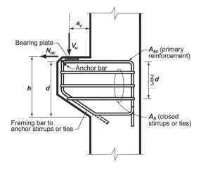
Fig. R16.5.1b—Notation used in Section 18.3.
