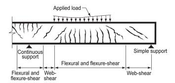
*Fig. R22.5.8.3—Types of cracking in concrete beams.*
