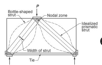
Fig. R23.2.1—Description of strut-and-tie model.
