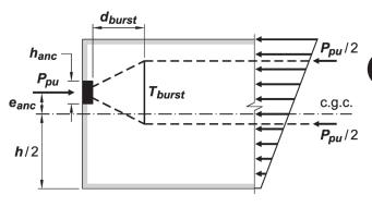
Fig. R25.9.4.3.1—Definition of terms used to define the general zone.
