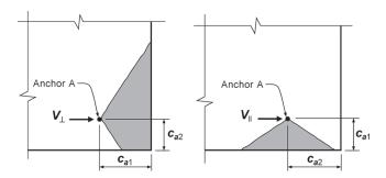
Fig. R17.5.2.1d—Shear force near a corner.
