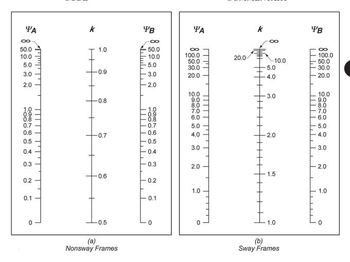
$\Psi = \text{ratio of } \Sigma(EII\ell_c)$  of columns to  $\Sigma(EII\ell)$  of beams in a plane at one end of a column
