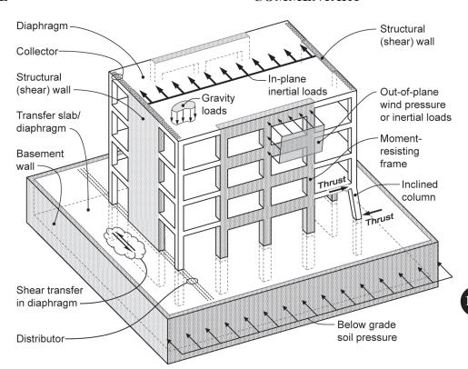
Fig. R12.1.1—Typical diaphragm actions.
