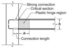
(b) Beam-to-column connection
