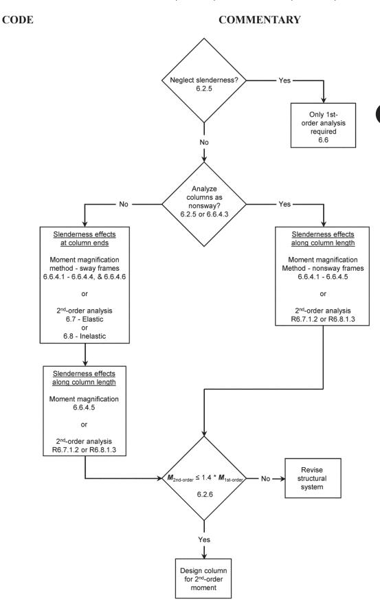
Fig. R6.2.6—Flowchart for determining column slenderness effects.
