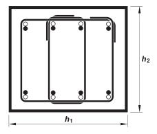
Direction 1:  $4A_b \ge 0.0015h_1s$ Direction 2:  $2A_b \ge 0.0015h_2s$ where  $A_b$  is the area of the tie
