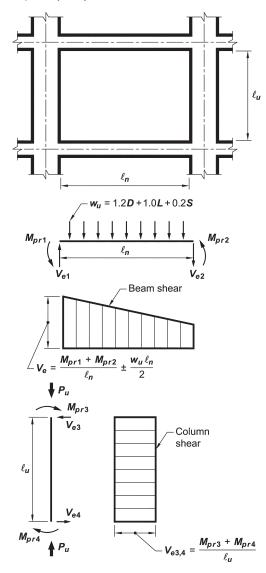
Fig. R18.6.5—Design shears for beams and columns.
