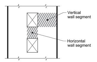
Fig. R18.10.4.5—Wall with openings.
