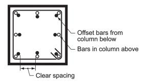
Fig. R10.7.5.1.3—Offset column bars.
