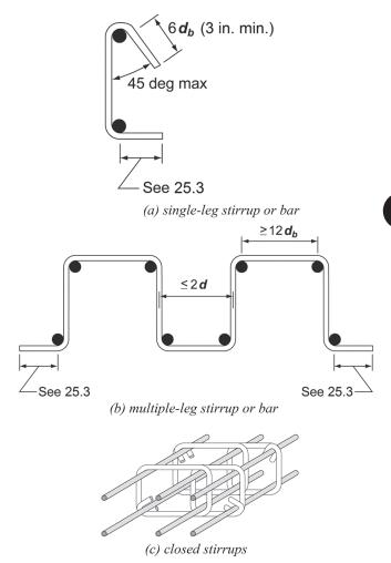
Fig. R8.7.6(a)-(c)—Single- or multiple-leg stirrup-type slab shear reinforcement.
