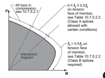
Fig. R10.7.5.2—Lap splice requirements for columns.
