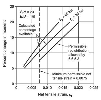
**Fig. R6.6.5**—Permissible redistribution of moments for minimum rotation capacity.
